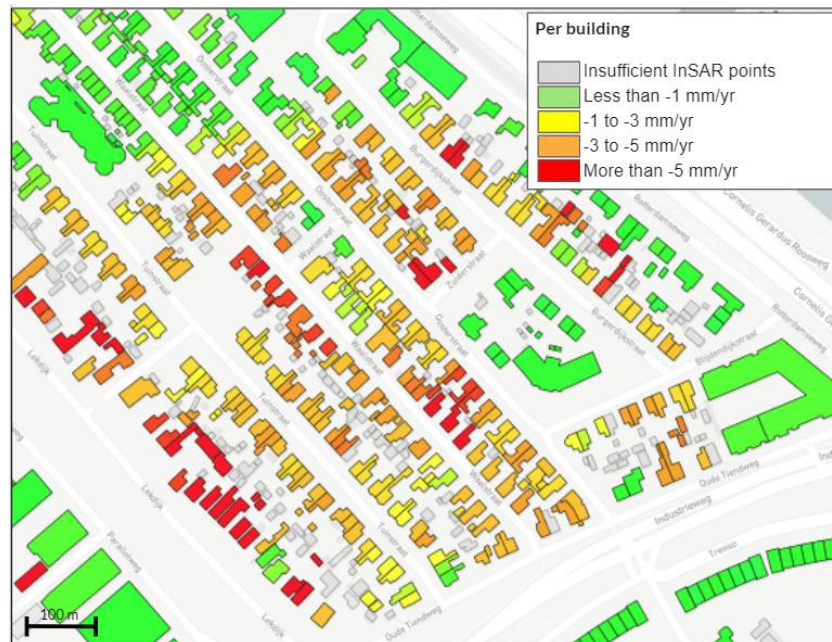
Figure 3: Average settlement rate per building, over the period 2009 to 2020, in a neighbourhood of Krimpen aan den IJssel. Settlement rates are variable across the area, to the north-west and south-east the houses are generally stable with displacements less than 1 mm/yr. However, in the centre, there are several houses subsiding at > 5 mm/yr.
