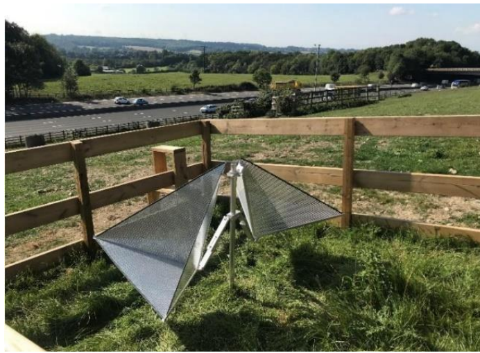
Figure 8: Installed trihedral reflector at Flint Hall Farm, M25 (Source: AECOM).
