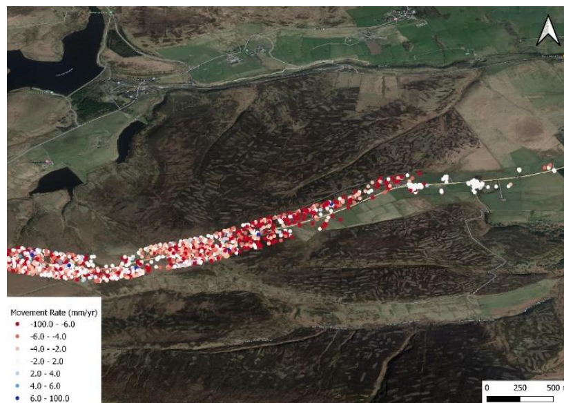
Figure 4: Example of high ground movement rates from PSInSAR data for a section of the A628 near Langsett associated with the Moorland areas visible in the image (InSAR data: SatSense; Map imagery: Google, 2022).
