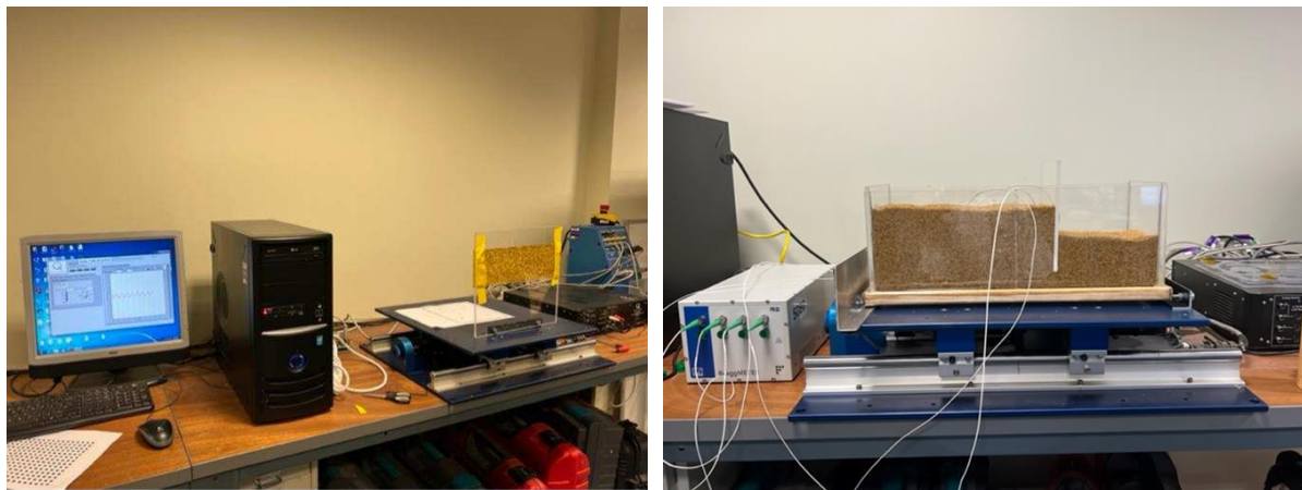
Figure 2a: LJMU 1g Quanser Shake Table II apparatus to the left, Figure 2b to the right model container, with wall and fibre cables embedded in the model, and FS 22 Interrogator.
