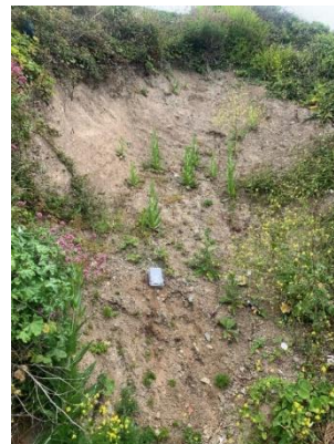
Figure 2: Sensor deployment on Connolly St slope, Cobh. Figure 3: Sensor deployment on Connolly St slope, Cobh.
