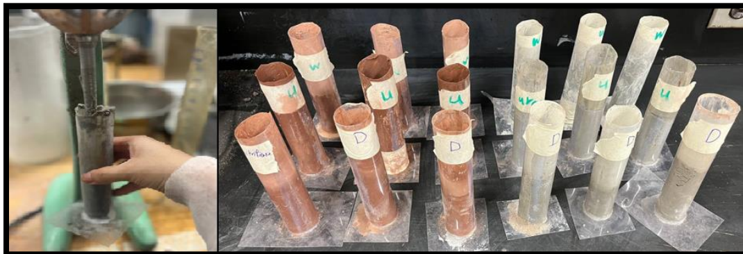
Figure 2. Left: DMM in the prepared mold, Right: Prepared soil samples
