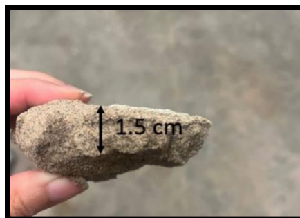
Figure 3. A portion of the sand dune stabilized by the spray method
