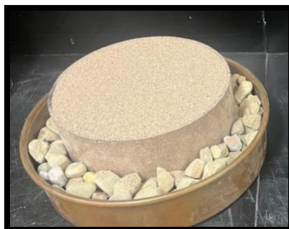
Figure 1. Sand dune samples prepared for the denitrification-MICP experiments (spray test) in the soil environment
