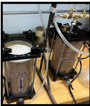
Figure 2. Sand column test specimens, (left: relatively aerobic, right: relatively anaerobic)
