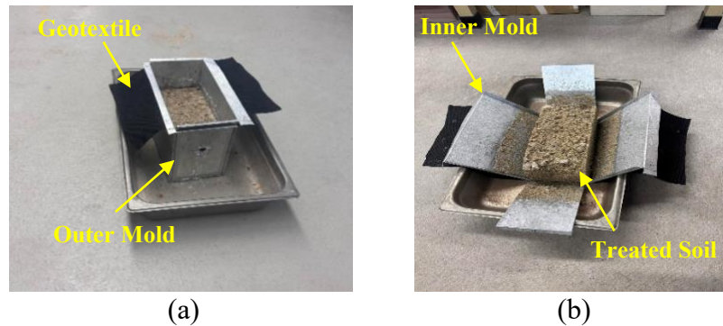
Figure 2. (a) MICP treatment block, (b) Dismantle mold and treated soil
