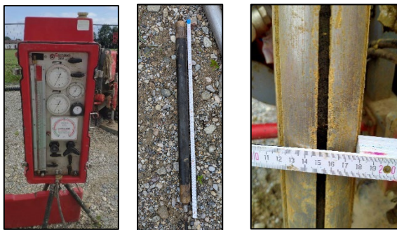
Figure 4. Menard control unit and Tri-cell pressuremeter probe Type G-AX with and without slotted tube.
