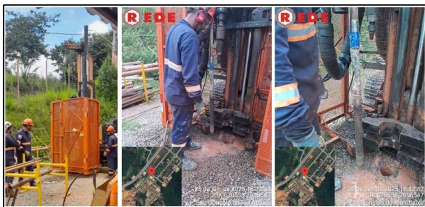
Figure 2. PMT Assay Preparation and Probe Positioning. - Source: REDE Engenharia.
