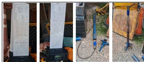
Figure 1. Pressure probe calibration process. Source: REDE Engenharia.
