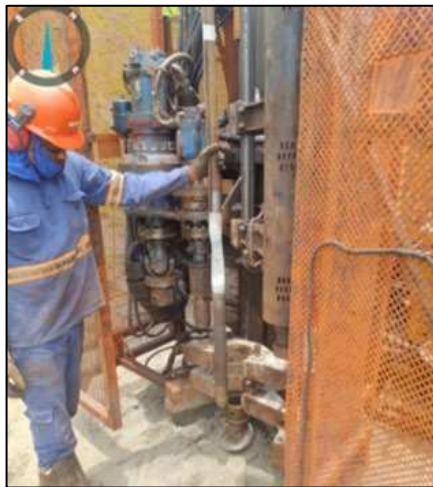
Figure 3. Hydraulic probe insertion for in-situ test. - Source: REDE Engenharia.
