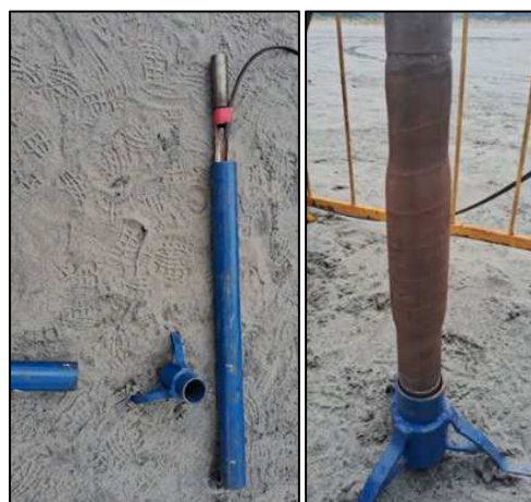
Figure 1. Volume loss and pressure loss probe calibration. - Source: REDE Engenharia.
