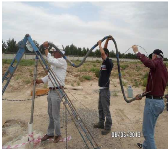
Figure 5. Conducting PS Logging test at site
