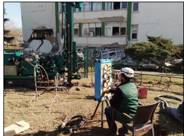
Figure 3. Pressuremeter test being conducted in study area
