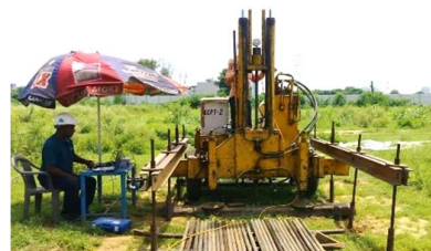
Figure 10. Cone Penetration Test in progress.
