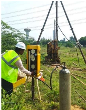
Figure 5. Pressuremeter Test in progress.
