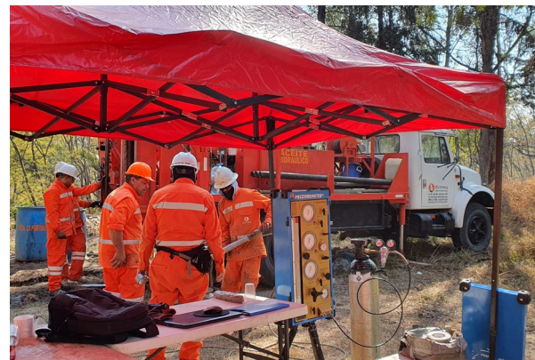
Figure 4. Performance of a pressuremeter test at site project
