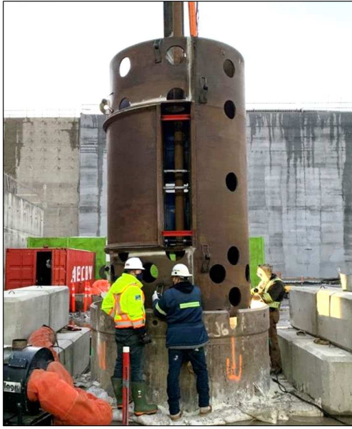
Figure 6. Site C lateral Osterberg load frame
