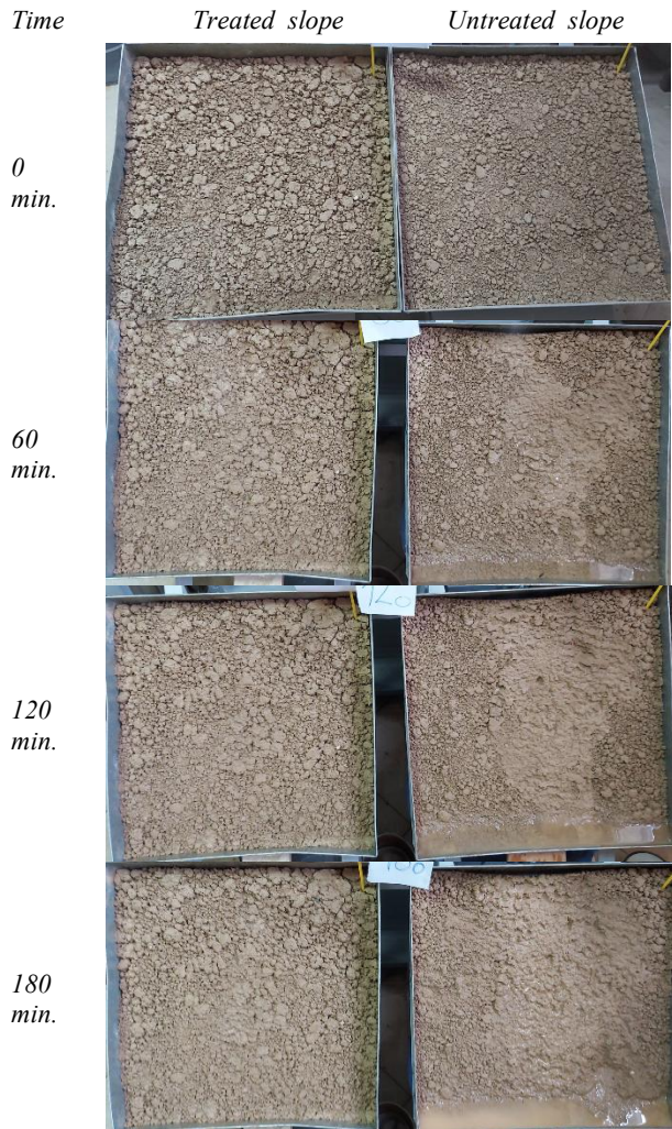
Figure 4. Experimental testing - erosion resistance test
