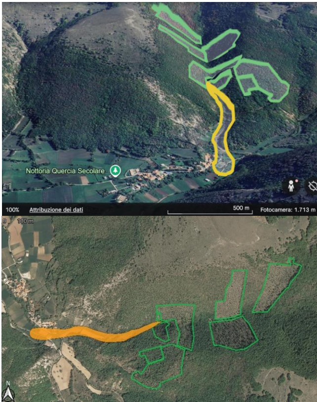
Figure 1. Google Earth (3D oblique view at top) and plan (at bottom) views of the study site with green polygons showing the cut areas and the orange polygon representing the debris flow area from the IFFI's database.
