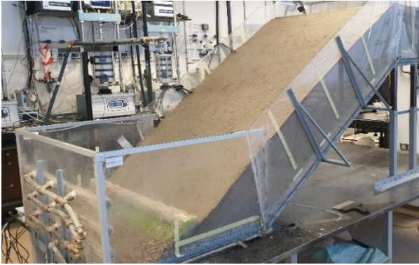
Figure 2. A 35° model built from uniformly-grained fine sand over a 5 cm thick layer of gravel.
