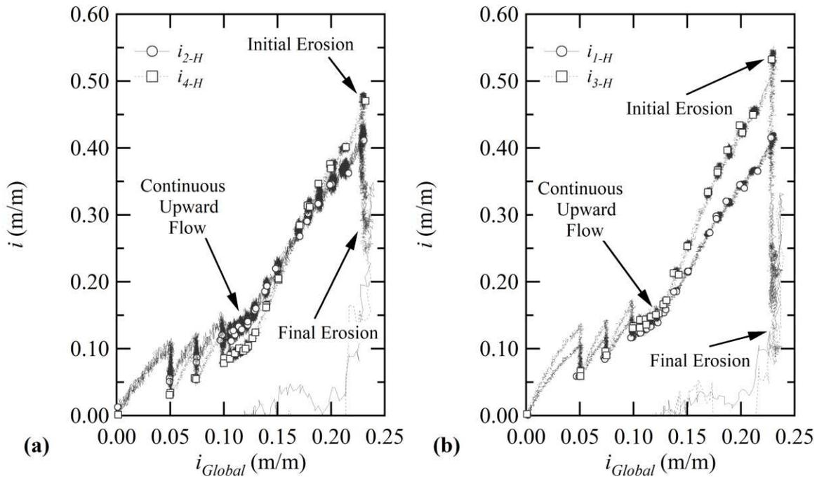
**Figure 5. Evolution of local and global hydraulic gradients: (a) left and (b) right sides of Model A.**
