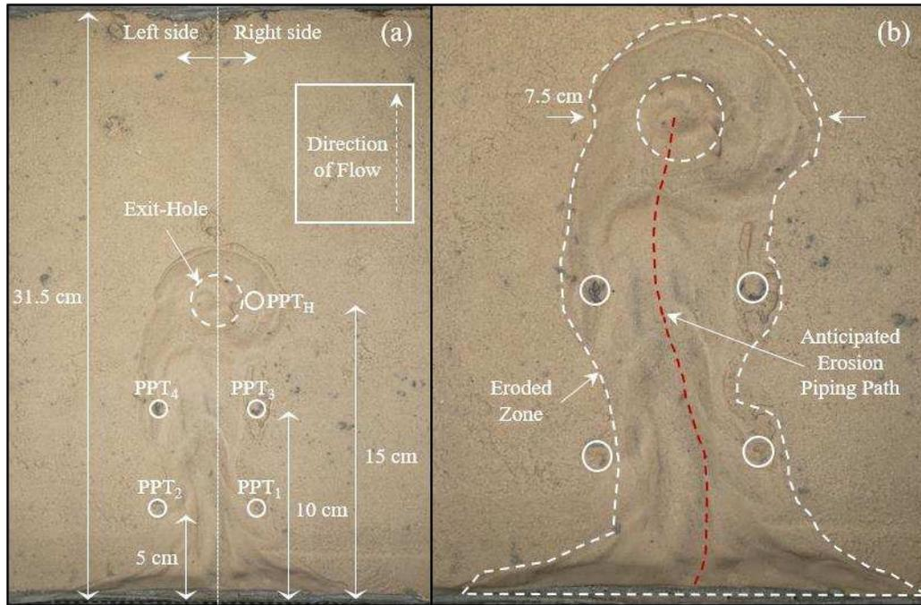
**Figure 3. Post-failure state of Model A: (a) total surface and (b) erosion zone.**
