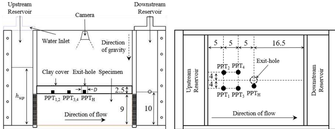
**Figure 1. Lateral and plan views of experimental setup (units in cm).**
