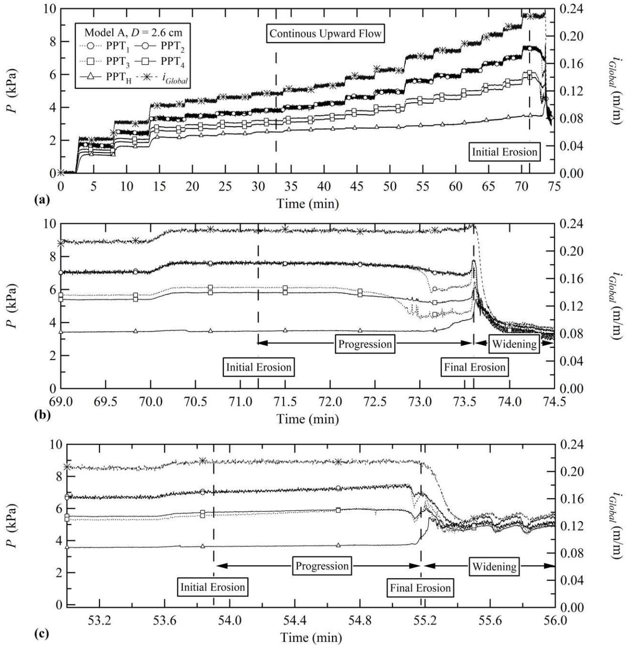
**Figure 4. Evolution of pressure readings: (a) total duration of test and (b) last increment of  $i_{global}$  in Model A, and (c) last increment of  $i_{global}$  in Model B.**
