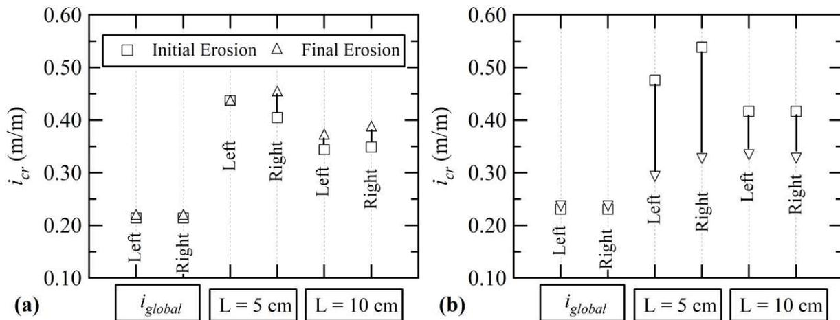
**Figure 6. Critical global and local hydraulic gradients: (a)  $D = 1.8$  cm and (b)  $D = 2.6$  cm.**
