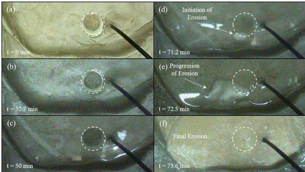
**Figure 2. Evolution of backward erosion piping in centrifuge model A.**
