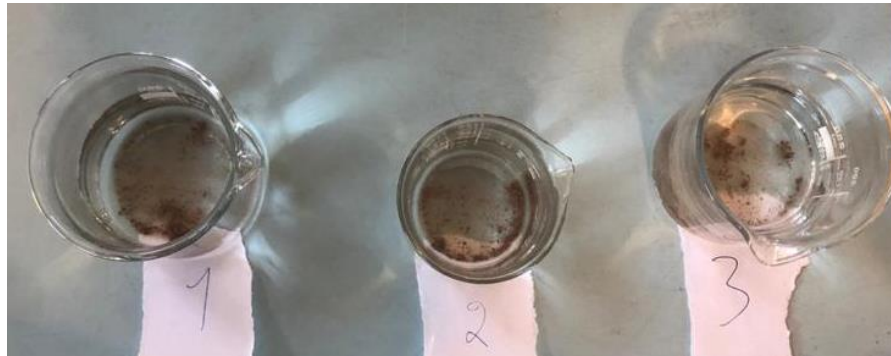
Figure 4 - Water samples collected during water seepage in the hole. Beaker 1 corresponds to the time when samples were first witnessed downstream (6 mins), beaker 2 is during the first collapse (13 mins) downstream and beaker 3 corresponds to the time before the failure of the weak zone (15 mins)
