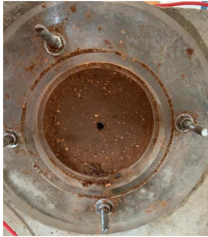
Figure 2 – Weak zone for the concentrated leak testing showing the 8 mm hole in the middle of the sand-clay mixture
