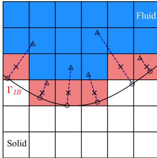
**Figure 1. 2D schematic view of the immersed boundary method including the IB cell centers (black cross), hit points (black circles), image points (black triangles), IB cells (red filled), fluid cells (blue filled), and solid cell (white filled). The immersed interface,  $\Gamma_{IB}$ , is the black curve.**
