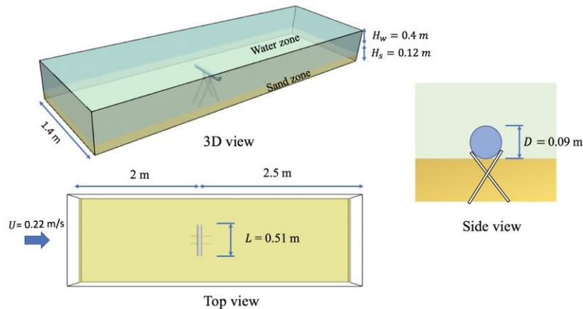
**Figure 3. Setup for the simulation of scour around a cylinder on a cradle.**
