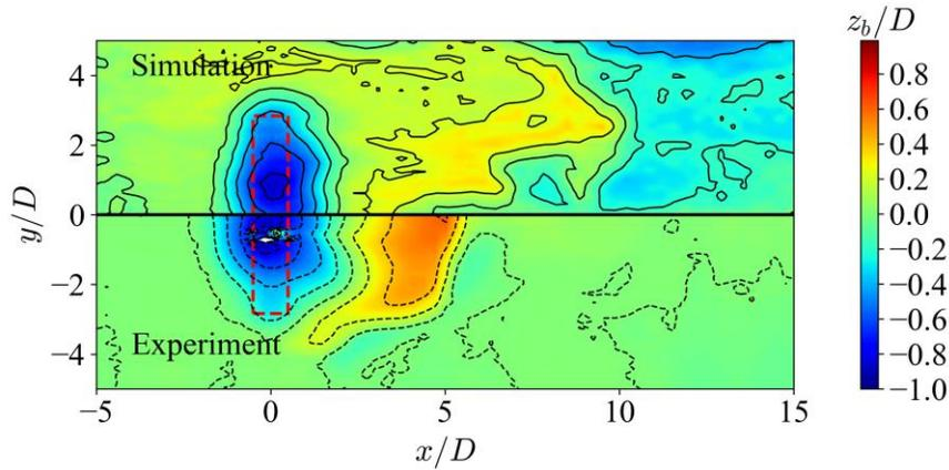
**Figure 4. Comparison of bed elevation at equilibrium for scour around a cylinder on a cradle. The upper panel is from the simulation and the lower panel is from the experiment.**
