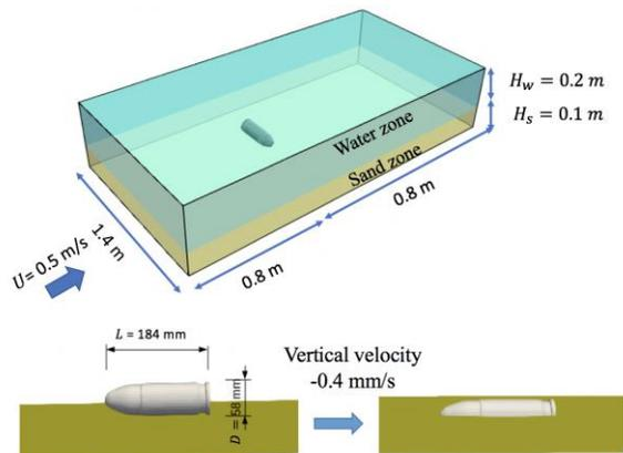
**Figure 5. Setup for simulation of scour around a munition sitting on a sediment bed.**
