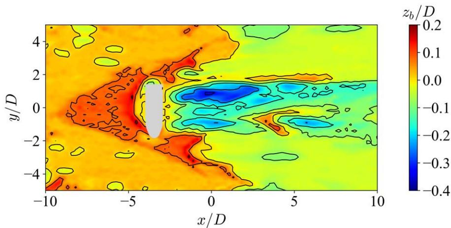
**Figure 6. Simulation result of bed elevation at equilibrium for scour around a mobile munition.**
