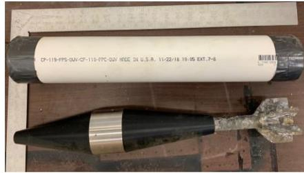
**Figure 2. Cylinder and the surrogate of a UXO.**
