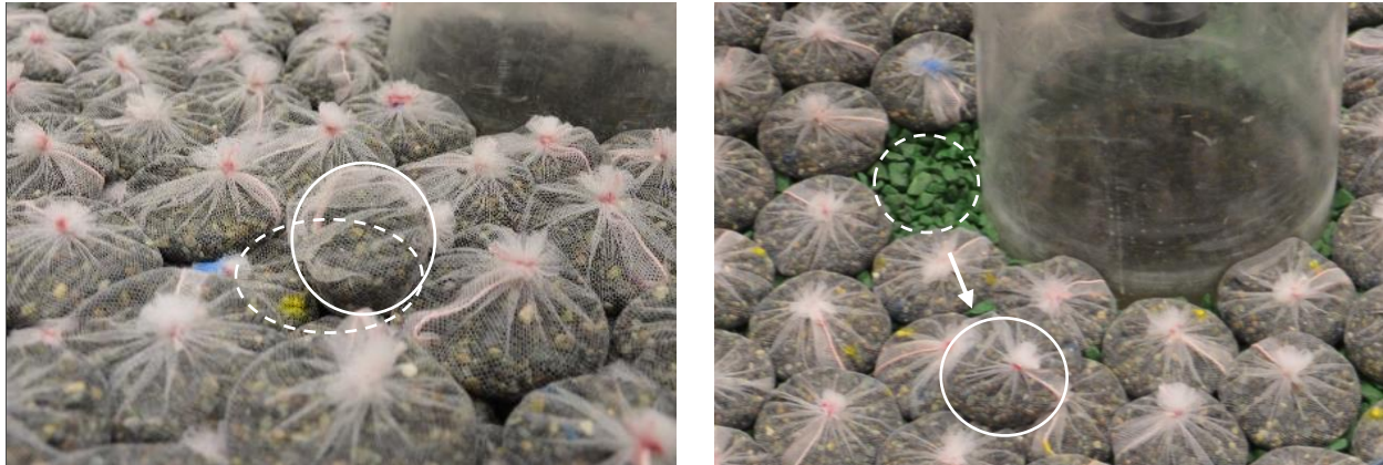
Figure 3: (left) Rolling over of a single mesh bag due to gradual residual displacement of filling material. (right) Instantaneous removal of a mesh bag element from the grid in a single layered arrangement.
