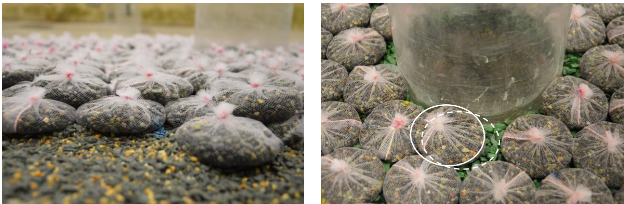
Figure 2: (left) Undermining of a mesh bag due to gradual removal of the base layer. (right) Reshaping of a single mesh bag by deformation of the filling material.
