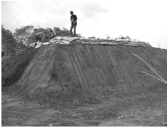
Fig. 16 – Simulation of load by dead weight
