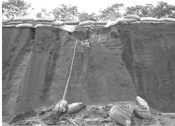
Fig. 19 – Erosion failure of trial embankment
