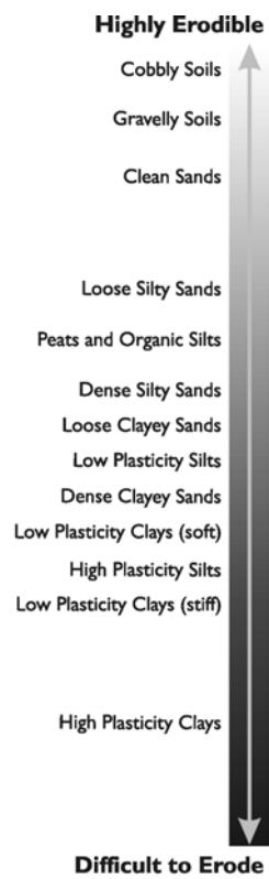
Figure 3. Erodibility scale for jet grouting systems, from Hayward Baker
