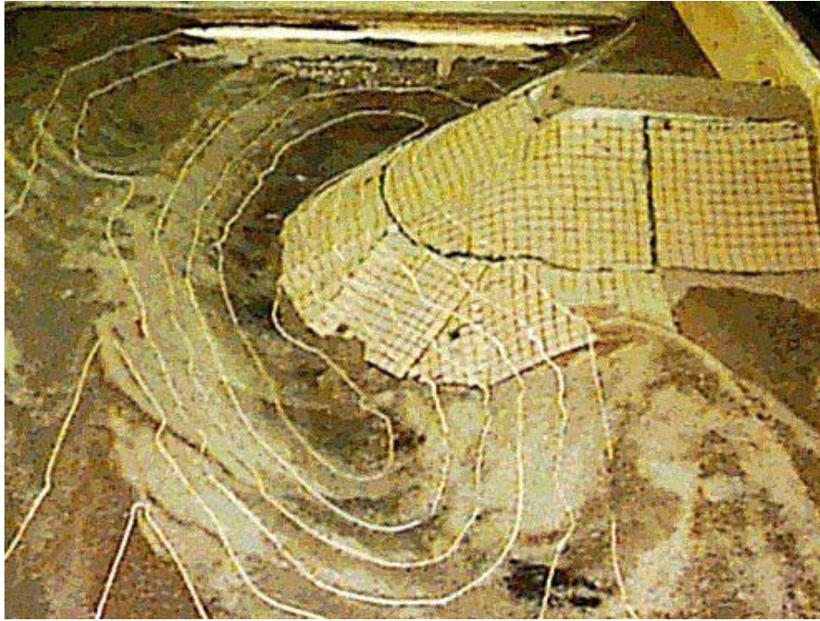
Figure 12 - Typical scour hole development for failed cable-tied block protection (Test 6), viewed from downstream. The failure was due to slumping of the fill material near the top of the embankment
