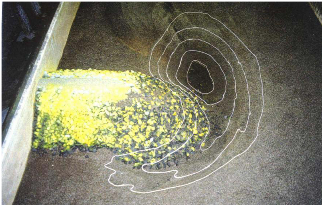
Figure 5 – Typical scour hole developed at an abutment (of no failure) with riprap protection, viewed from downstream
