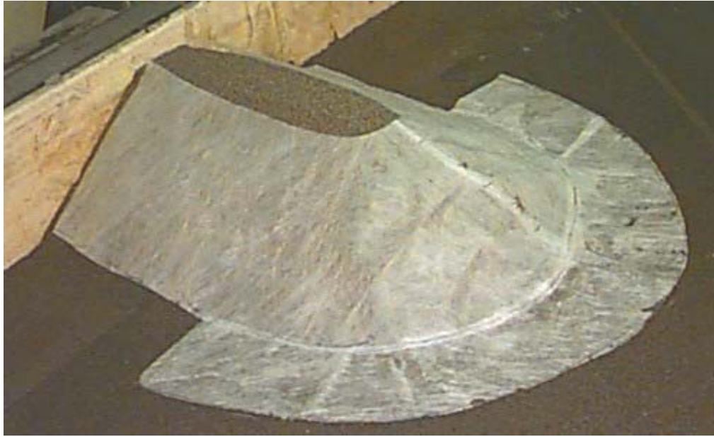
Figure 4 – The filter fabric placed over the sand embankment ready for placement of cable-tied blocks
