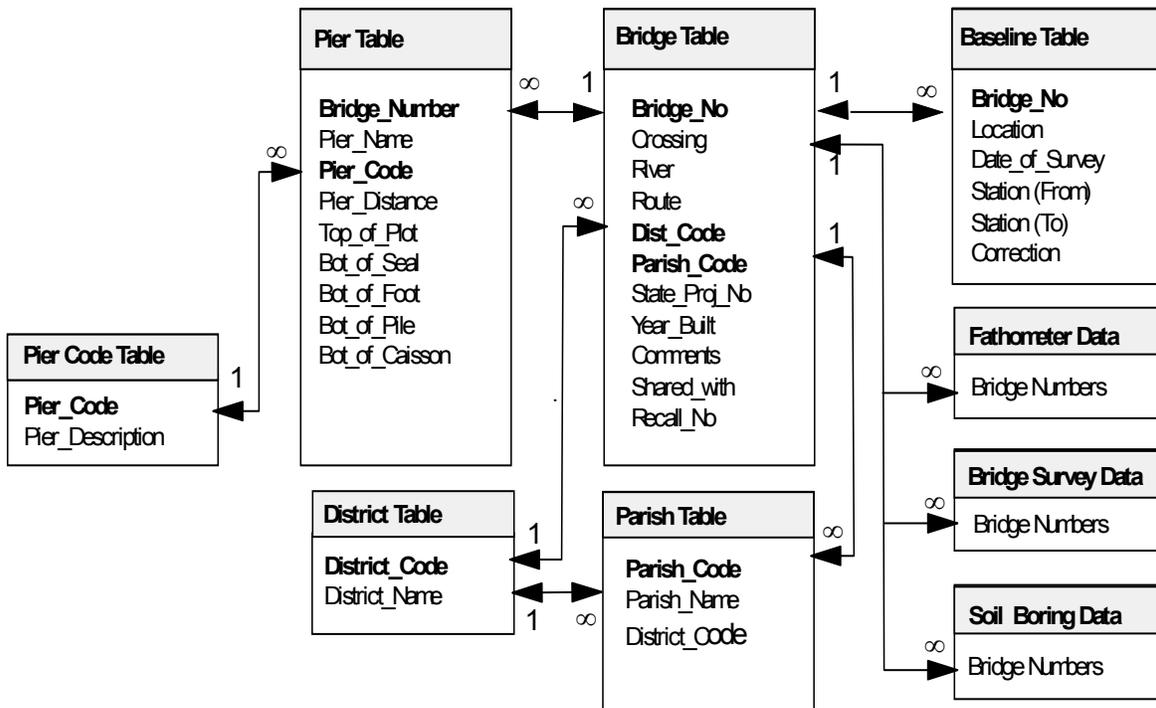
Figure 1. Data types and structure of the database
