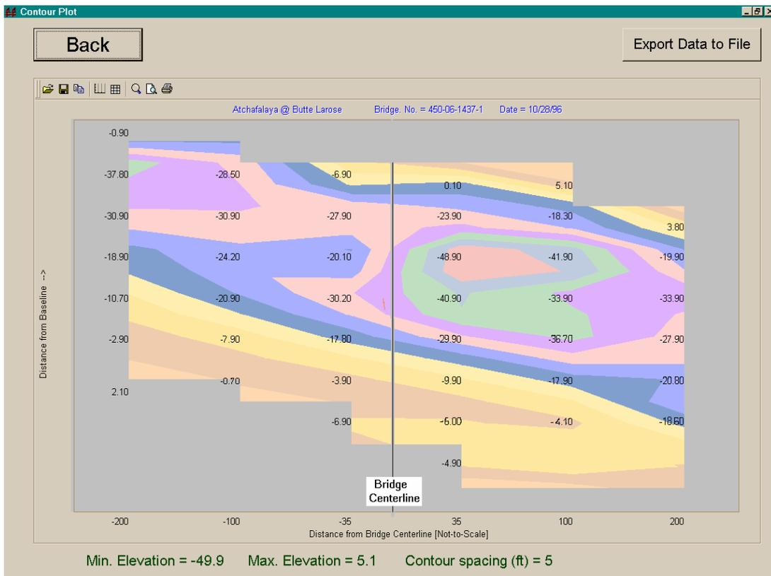
Figure 10. View of contour plot in the database program
