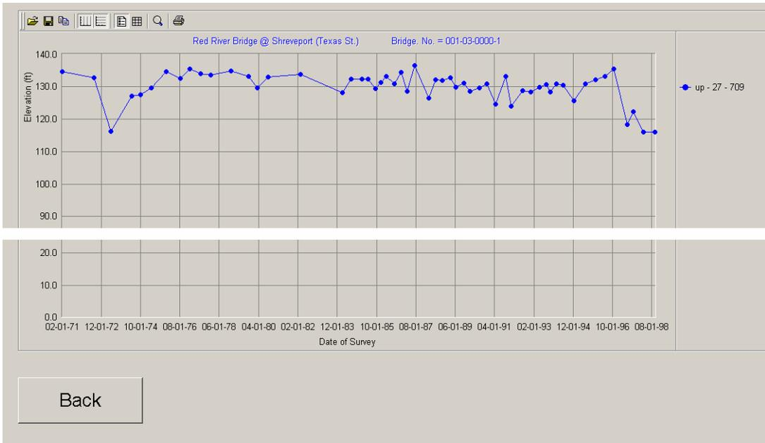
Figure 9. Tine plot showing the change of elevations near the pier at location shown in figure 8
