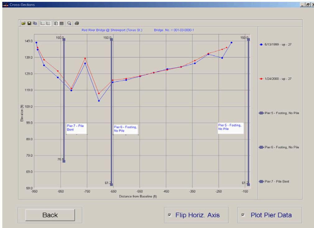
Figure 7 Cross-section plots for several dates at bridge downstream
