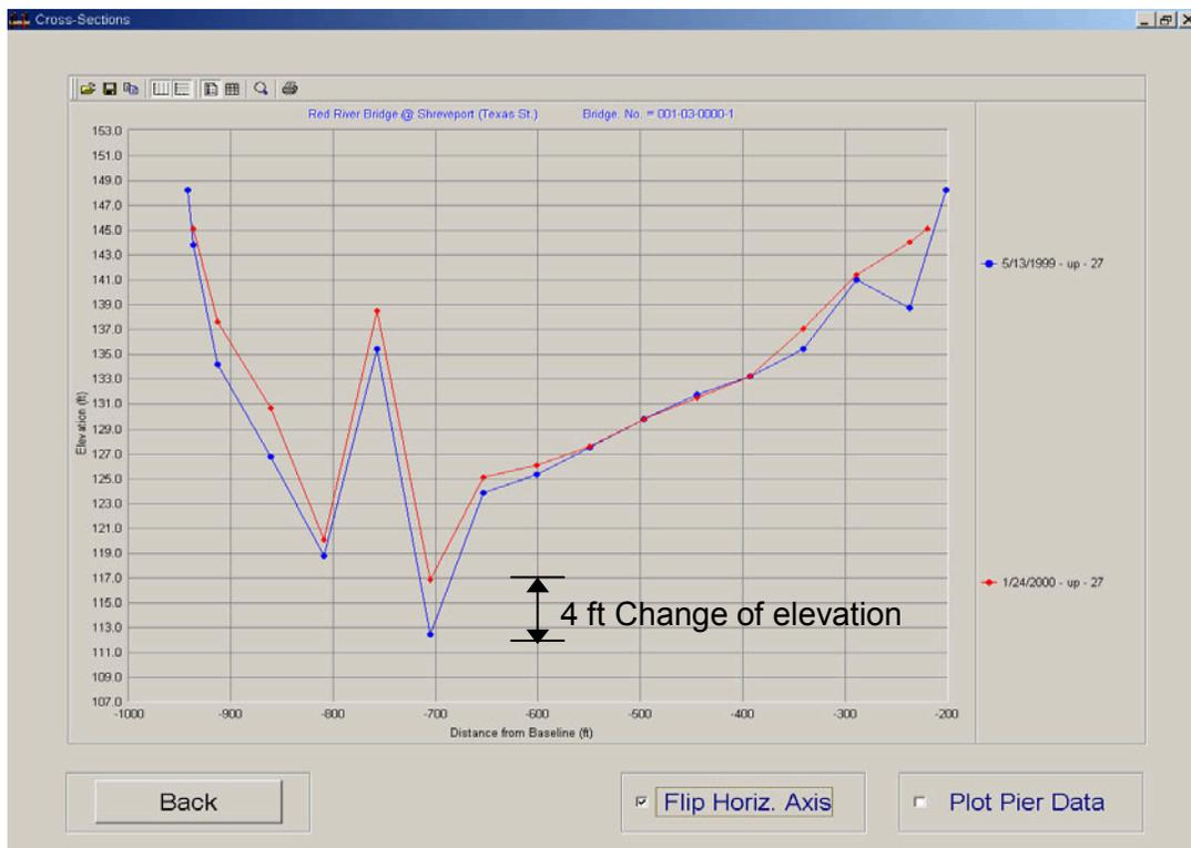
Figure 8. Detail of Figure 7 showing elevation changes at two consecutive fathometer readings
