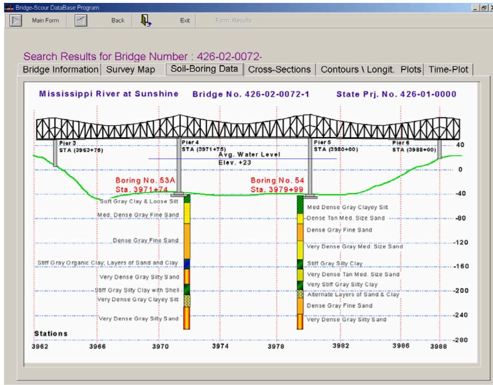
Figure 5. Schematic of the bridge structure showing soil boring locations and data
