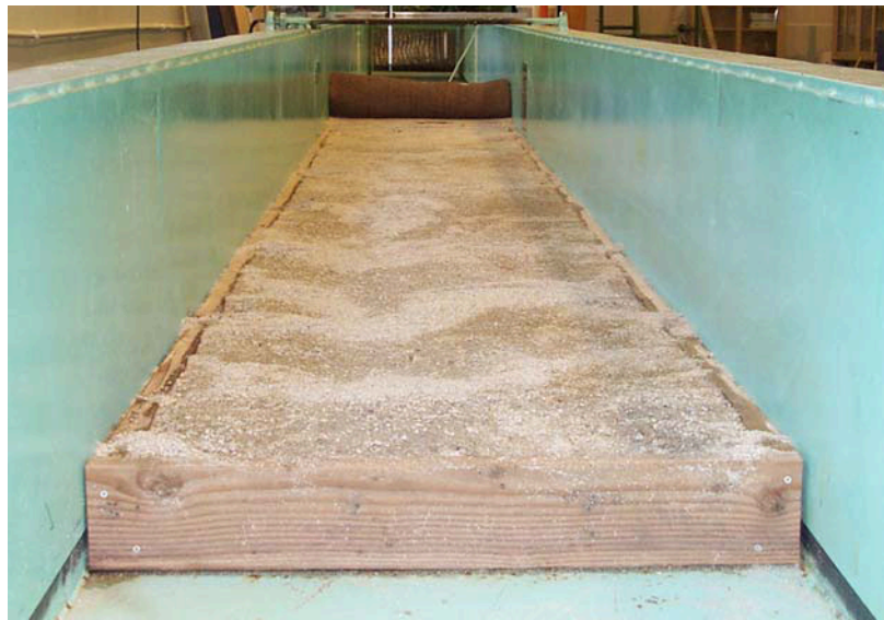
Figure 8. Soil Test Section within Flume
