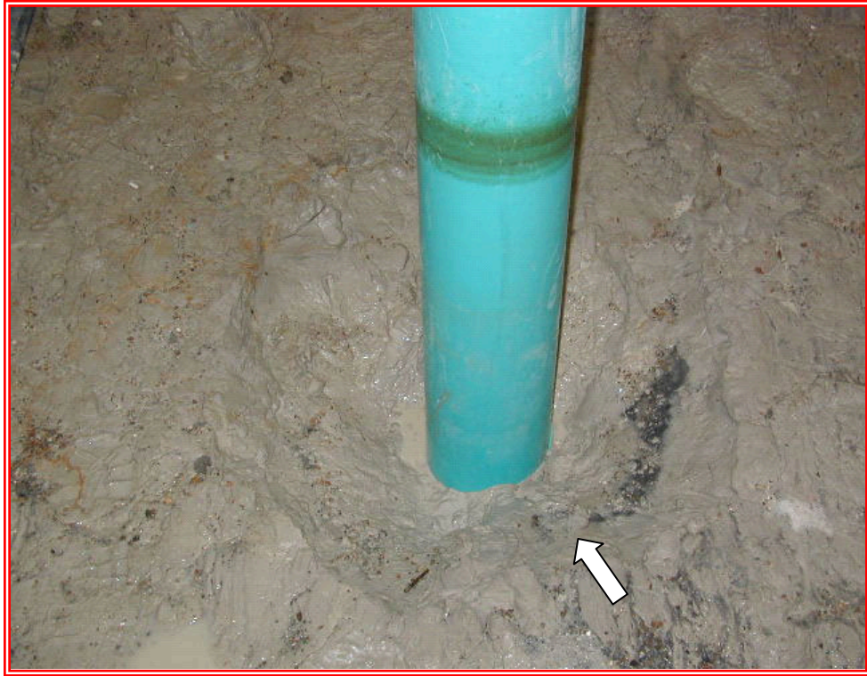
FIG 11 Scour Hole Geometry for Test 3
