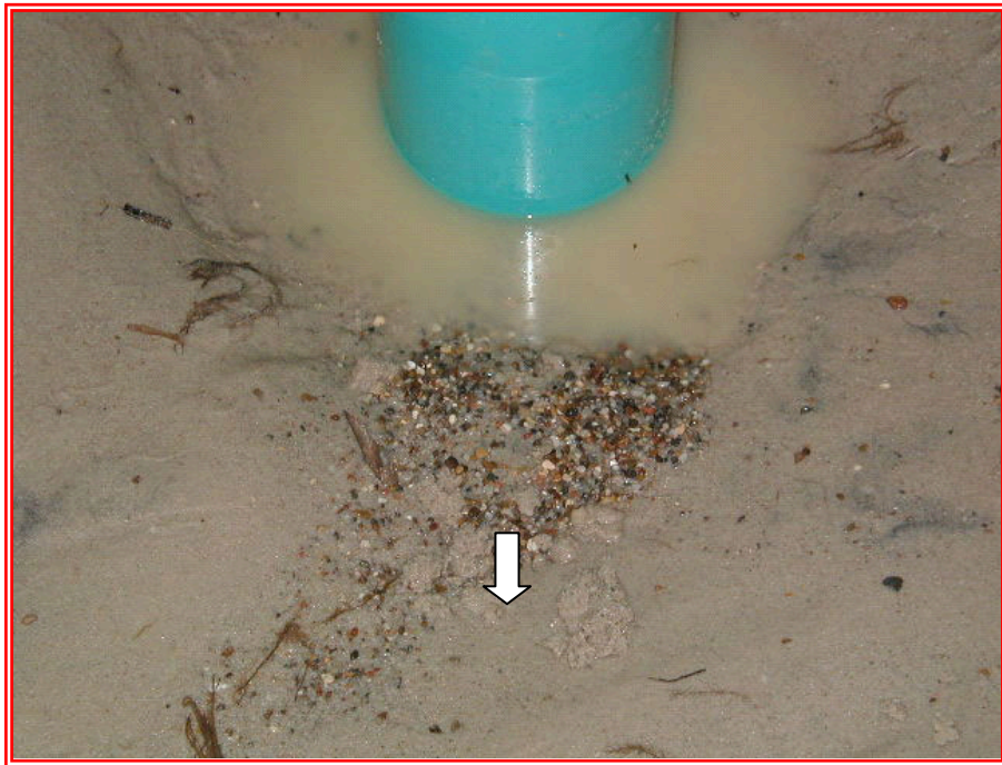
FIG 9 Coarse Particle Deposition in Test 2
