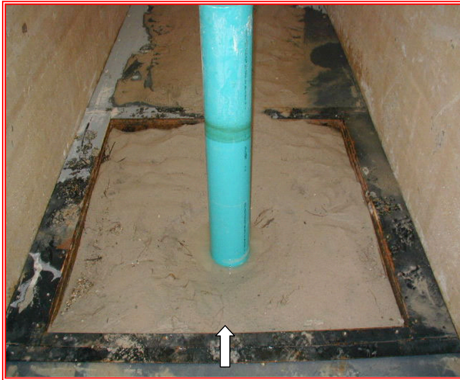
FIG 5 Scour Hole Geometry for Flume Test 1
