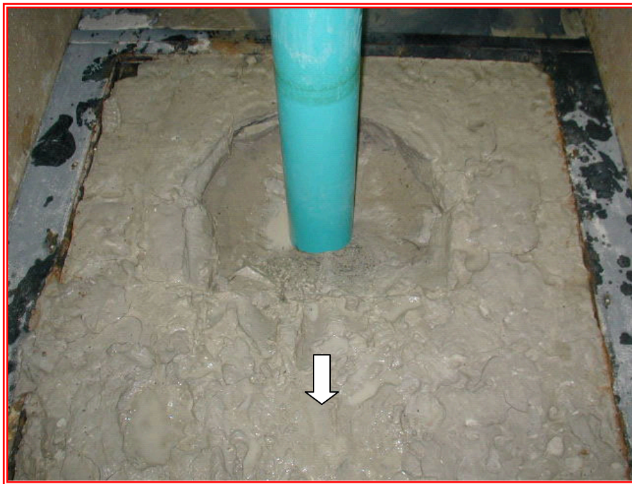
FIG 18 Back View: Scour Hole Geometry for Test 6
