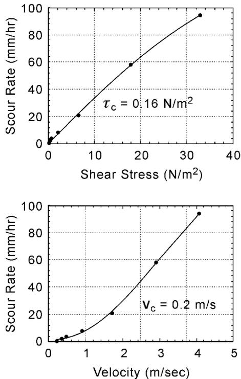
Fig. 6 Erosion Function for a soil sample taken near Pier 27E of the Existing Woodrow Wilson Bridge (11.2 – 11.7 meters depth) : a) Scour Rate vs. Shear Stress, b) Scour Rate vs. Velocity
