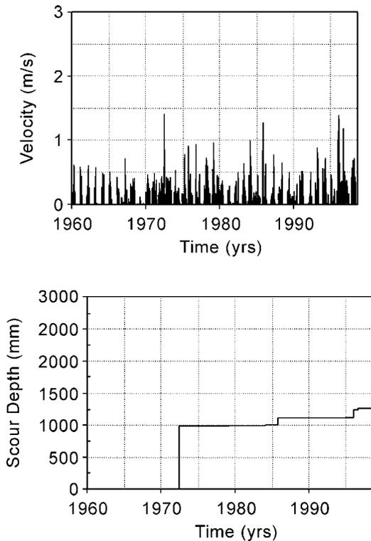
Fig. 10 Velocity Hydrograph and Predicted Scour Depth vs. Curve for Pier 27E of the Existing Woodrow Wilson Bridge
