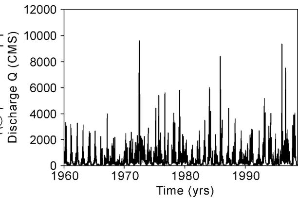
Fig. 3 Discharge Hydrograph at Woodrow Wilson Bridge (01/01/1960-09/31/1998)
