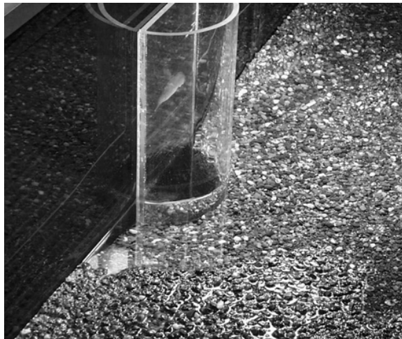
Fig. 2 - Side view on half-cylinder to visualize scour progress at various times t , for h_o=0.15 m, d_{50}=0.045 m, \sigma=2.2 and F_d=2.5 . Flow direction from bottom to top.
