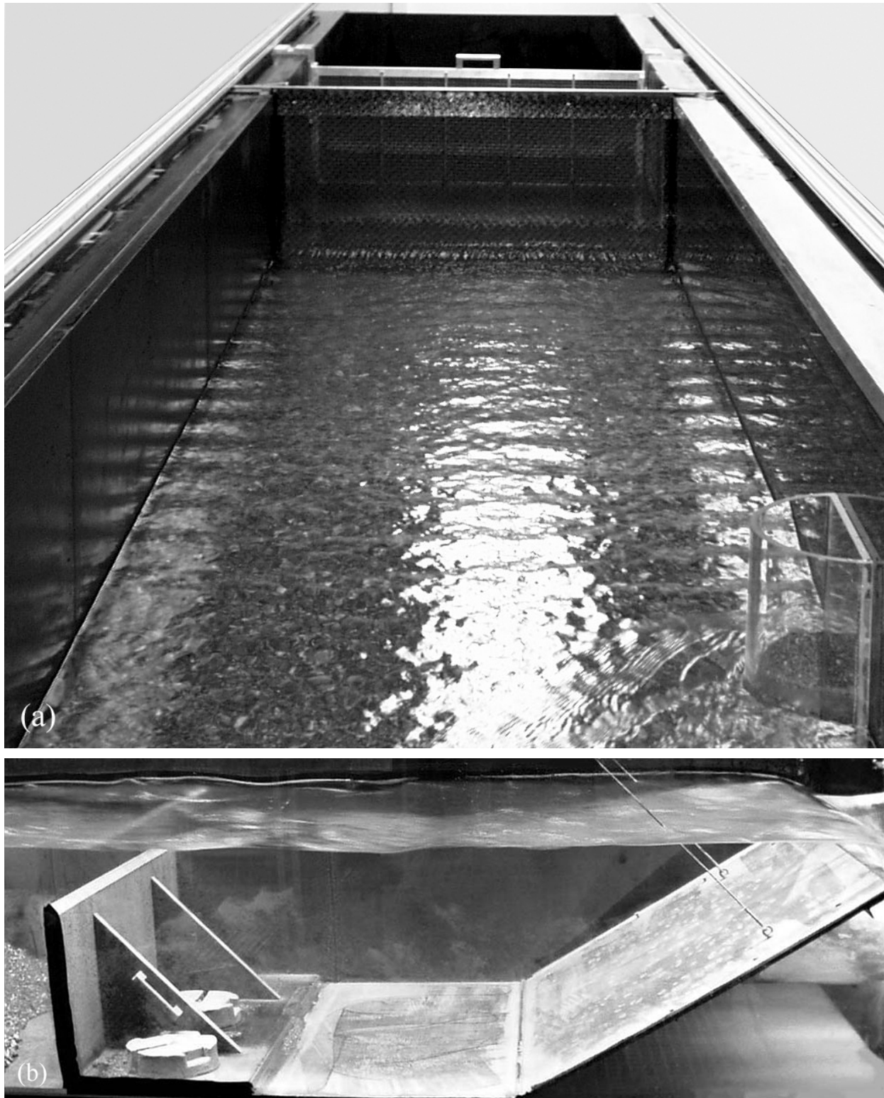
Fig. 1 - VAW scour channel (a) Upstream view with half-cylinder at glass wall, (b) Downstream view with submerged weir and flap gate.
