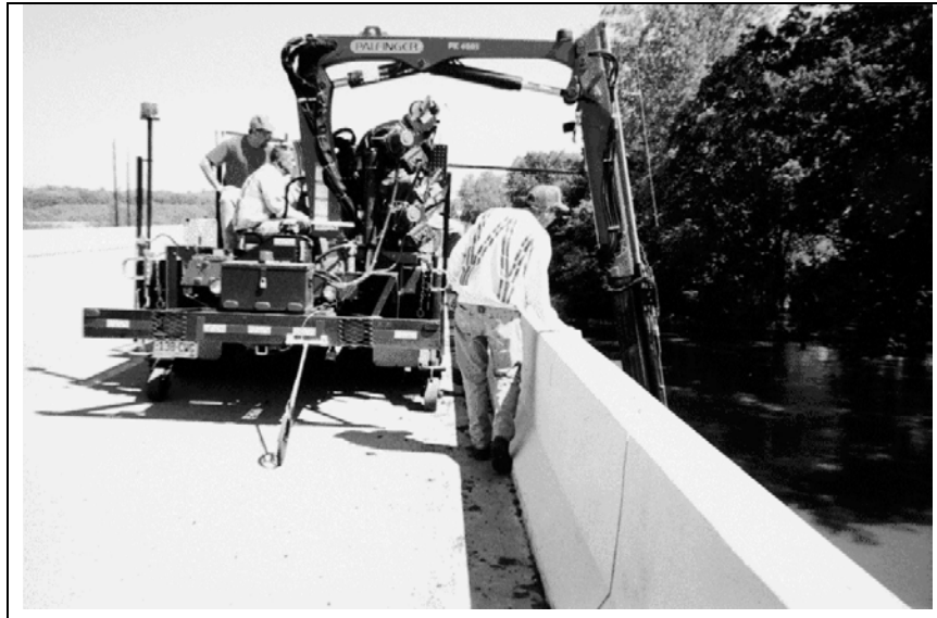
Figure 6. Collecting cross section data while driving the truck across the bridge.
