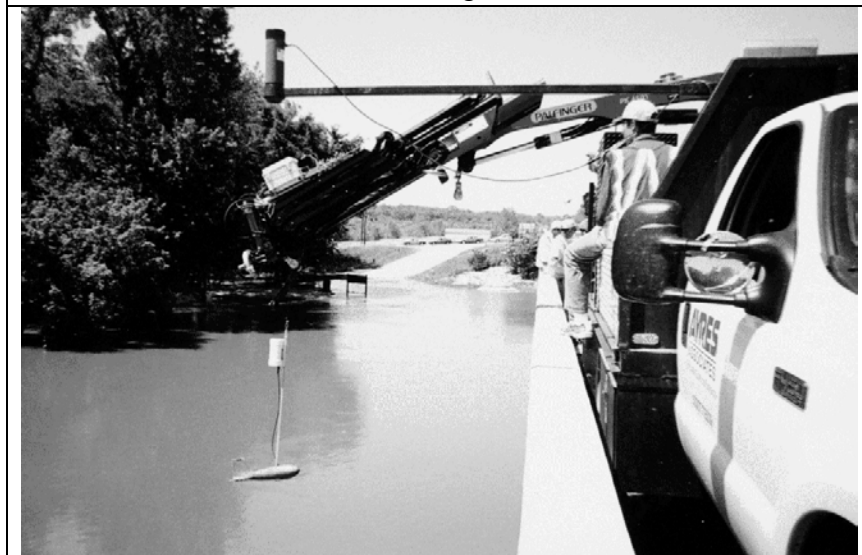
Figure 7. Wireless sonar in a sounding weight.
