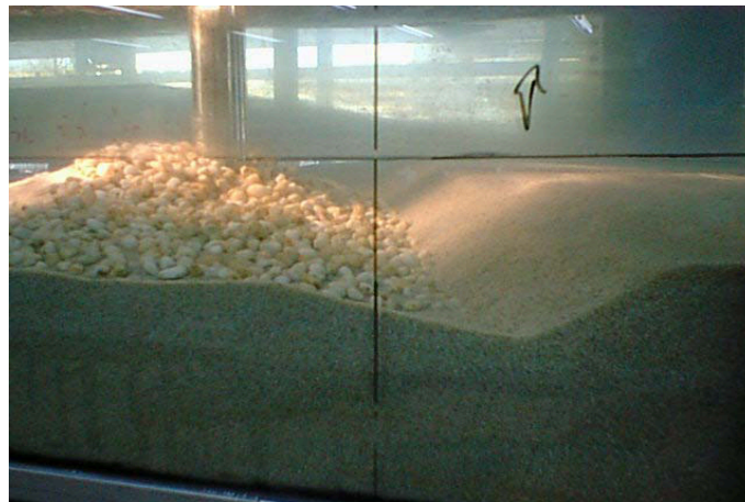
(b) Formation of riprap mound around pier (flow from right to left)
