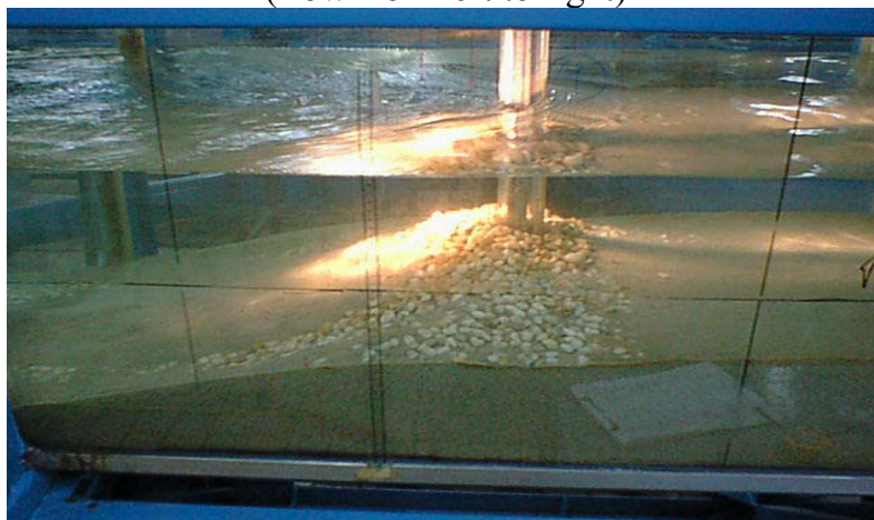
(c) Remains of the riprap mound after subsidence of the second flood (flow from right to left)
