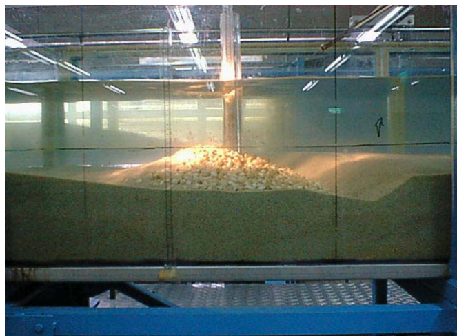
(b) Formation of riprap mound around pier (flow from right to left)
