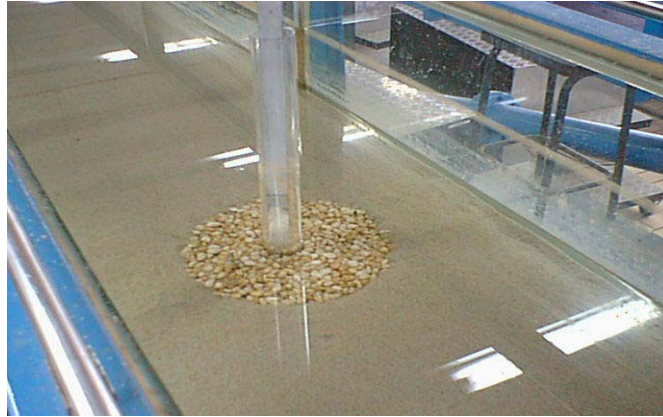
(a) Riprap layer at the commencement of test
