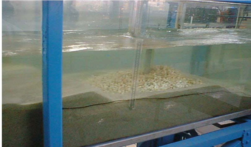
(a) Dune from second flood approaching the riprap mound (flow from left to right)
