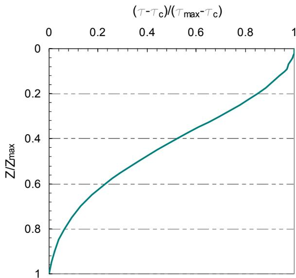
**FIG 3** Normalization of Shear Decay Curve
