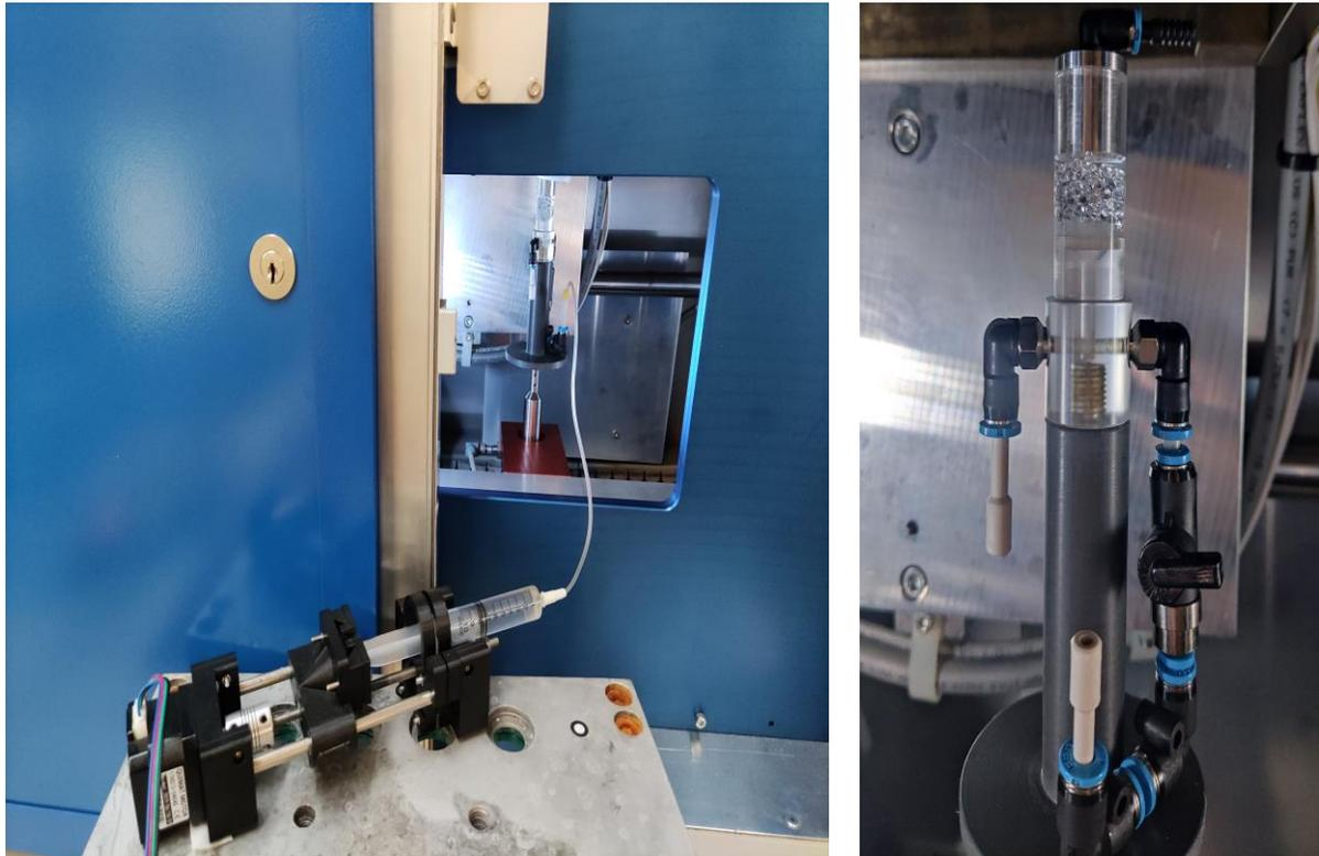
Figure 1: Syringe pump (left) connected to the sample holder (right) in the CT scanner.
