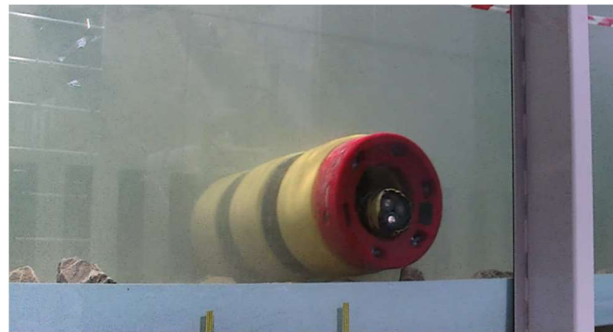
Figure 5. Standard cable-CPS product rolling over a rock pinnacle.
