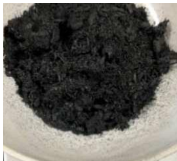
Figure 6. Carbonized material obtained by dry distillation gasifier
