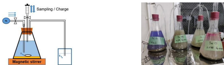
Figure 1. Diagram of the experimental setups (left). Photo of the actual test cases (right).
