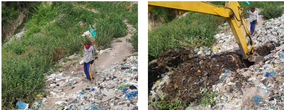
Figure 3. Placement of flag markers at a sampling point (left). Excavation of waste samples at a marked sampling point (right).
