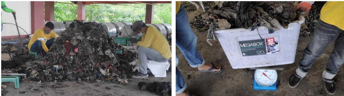
Figure 5. Sorting of coarse fraction (left). Weighing of soft plastics sorted from coarse fraction (right).
