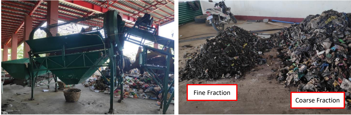
Figure 4. Trommel used to separate the fine fraction from the coarse fraction (left). Fine and coarse fractions after separation by the trommel (right).
