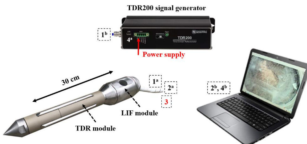
Figure 6. Configuration of the detection system based on the penetrometer
