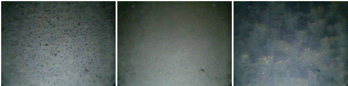
Figure 5. Images captured at depths 10, 14, and 18 m (from left to right) at location A1, lying in low, medium, and high permeability zones, respectively
