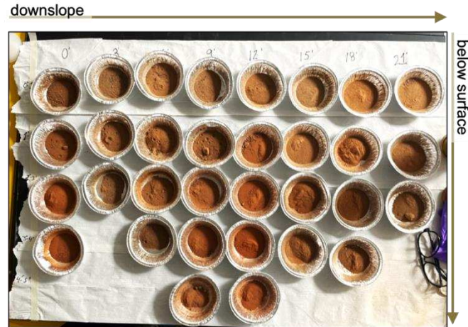
Figure 1. Soil Samples were collected from the slope at varying length and depth intervals.
