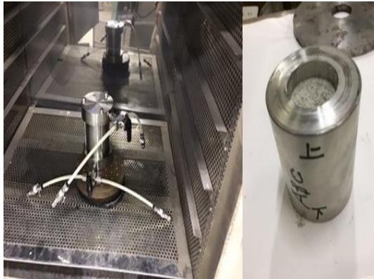
Figure 3. Steel mold used in Testing program (B)
