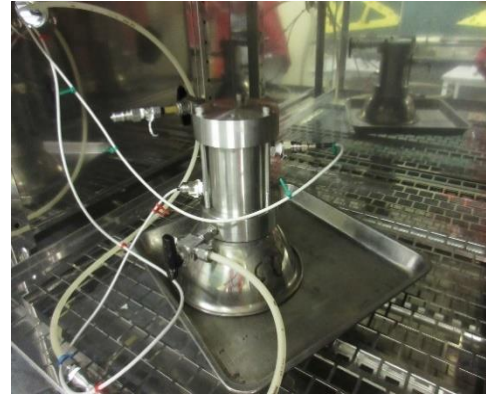
Figure 4. Steel mold installed pressure sensors
