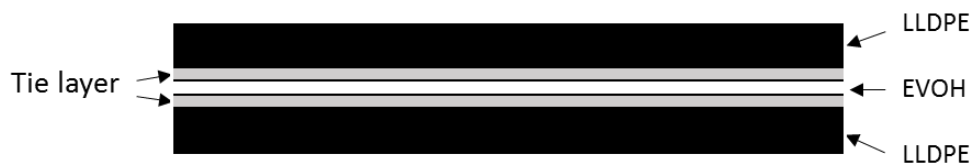
Figure 2. Schematic of EVOH geomembrane with LLDPE outer layers
