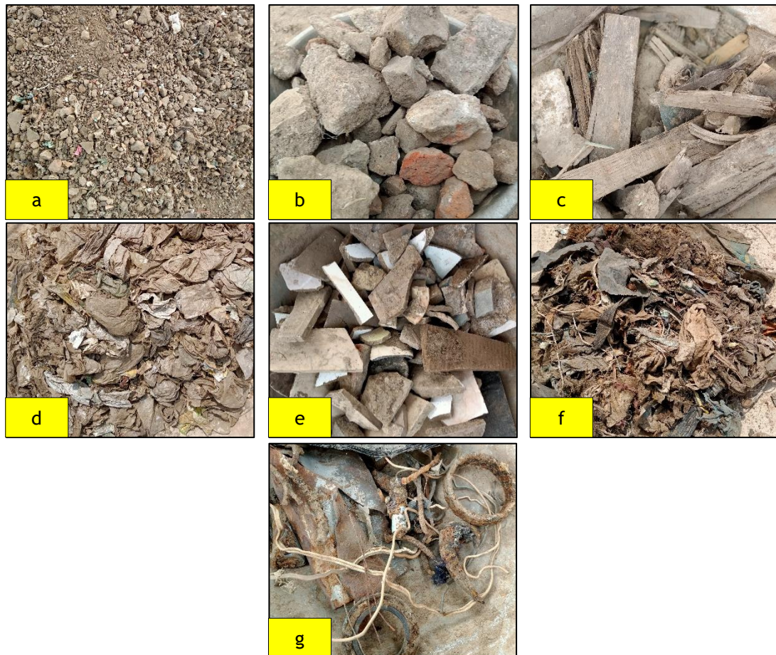
Figure 5. Composition of excavated legacy waste by manual sorting: a) fine fraction (<13.2mm); b) C&D fraction; c) wood; d) plastic; e) ceramics; f) textile; g) metal
