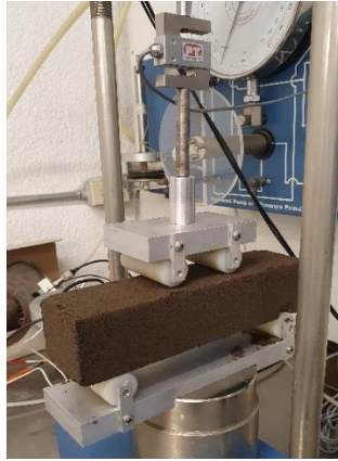
Figure 3 Bending beam test equipment
