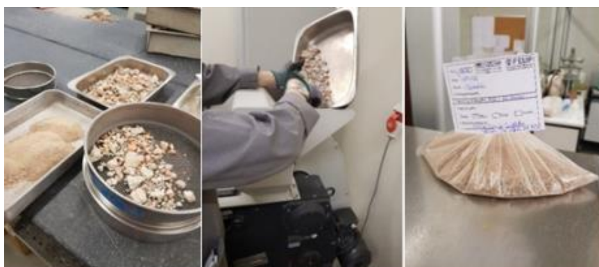
Figure 5. Determination of water soluble sulphate content
