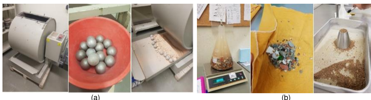
Figure 4. (a) Los Angeles method; (b) Particle density and water absorption test
