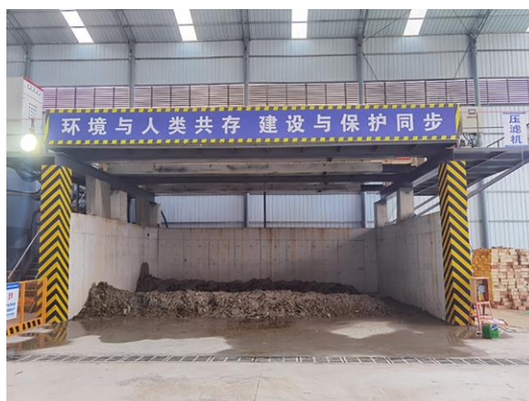
Figure 8. Filter press dewatering of the slurry
