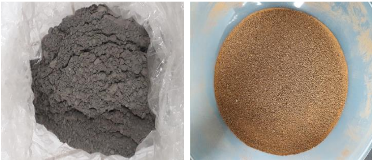
Figure 2. Coffee husk ash (CHA) used for the study (left). Clay soil passing sieve No. 4 (right)
