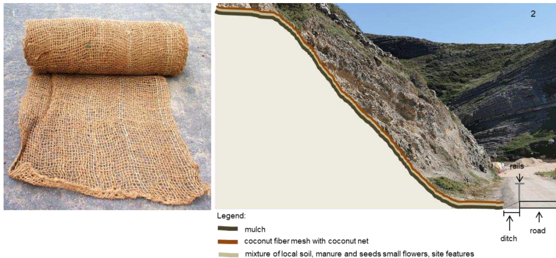
Figure 3. (1) Example of a coconut fiber mesh (Ecosalix, 2022) (2) Schematic cross section of the Vale da Anta slope with vegetated cover to promote stabilization of the fault zone
