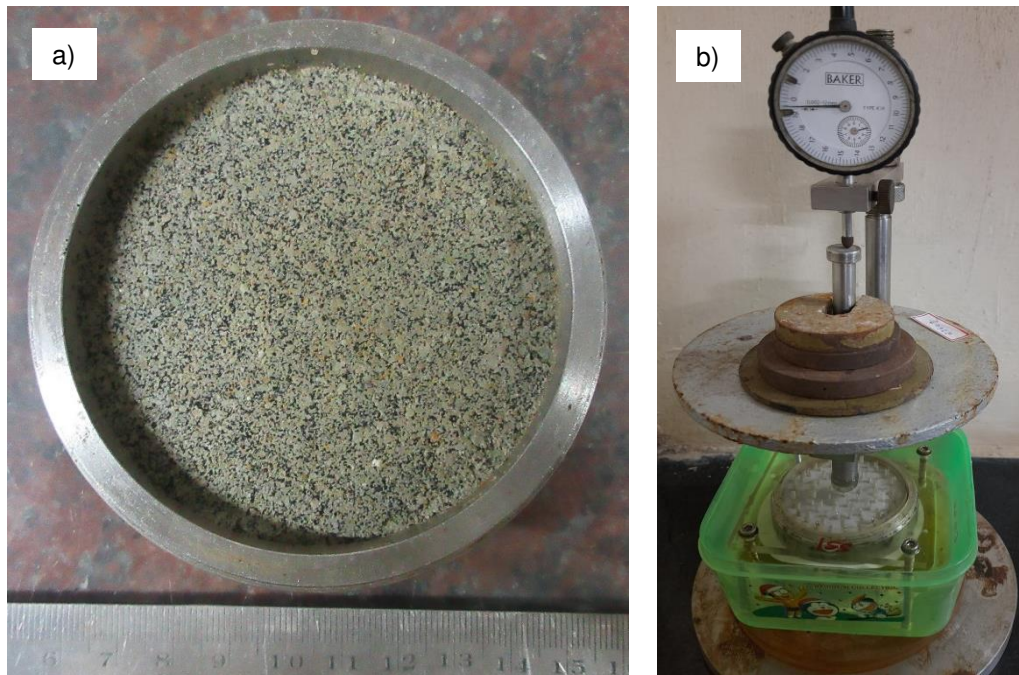
Figure 1. (a) Top view of compacted RC5 specimen and (b) swell setup
